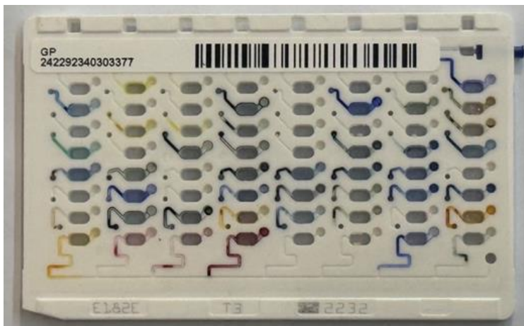
Figure 2. Identification card of the VITEK 2 compact system used for biochemical profiling of the bacterial isolates. The cassette contains a range of micro-wells containing dehydrated substrates that generate colorimetric signals upon inoculation and incubation, enabling automated identification of Aeromonas salmonicida in the VITEK 2 compact system.
